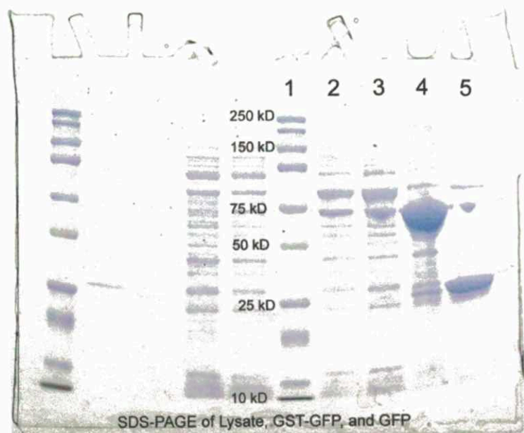
Figure 19: Photograph of SDS-PAGE result. Lane 1 – Marker Lane 2 – Induced lysate Lane 3 – Flow through Lane 4 – Resin bound fusion protein Lane 5 – Purified GFP
